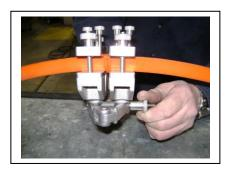
4. After you have removed the heated wand and tightened the thumb bolt let stand for approximately 5 minutes before removing from pliers. Continue to allow cooling for another 10 minutes.
